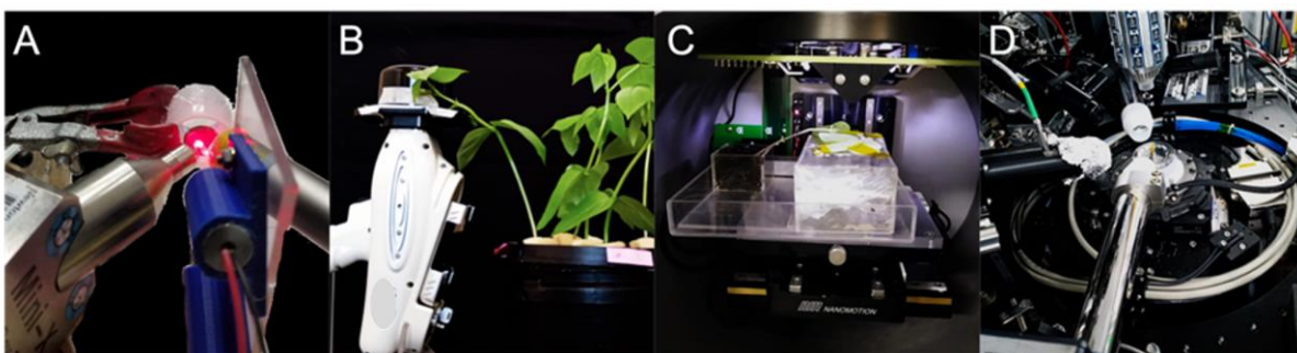
Fig. 1. X-ray fluorescence setups and geometries in laboratory and synchrotron beamline.
